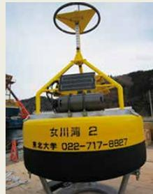
■ Building a real-time observing system for marine environment
