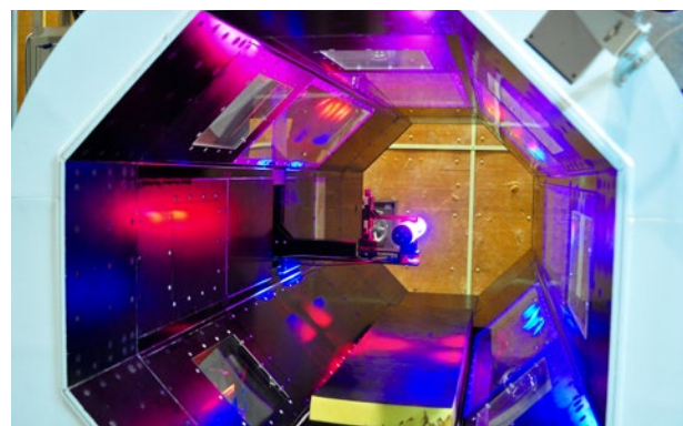
A cylinder is readied for a wind tunnel test by calibrating the position sensor on the test section of the Magnetic Suspension and Balance System, which can levitate objects for aerodynamic analysis.
