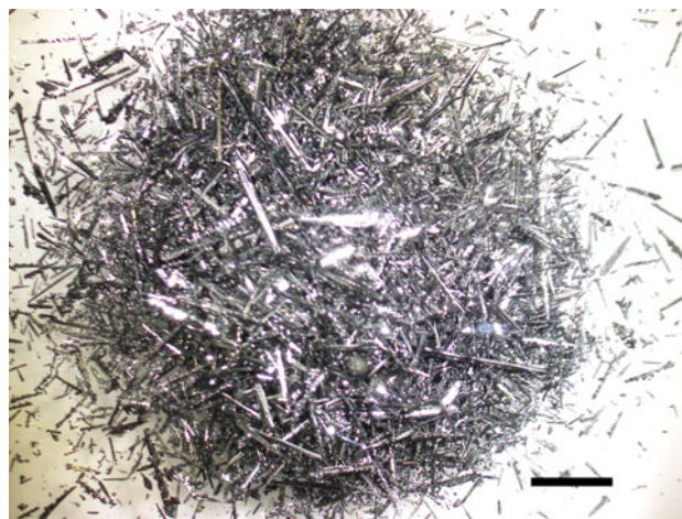
Fig. 1 Electrolysis of silver nitrate generates shiny black crystals of silver (III) oxide ( \text{Ag}_2\text{O}_3 ) clathrate. Platinum electrodes were submerged in 1-M silver nitrate solution and electrolysis was performed using 5 V for 15–30 min. Approximately, 2.8% of the silver was recovered around the anode. Scale bar represents 5 mm
