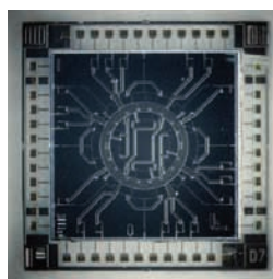
Electrostatically levitated rotational gyroscope
